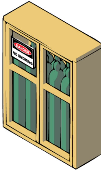
Figure 2-6: Compressed Gas Cylinder Storage
