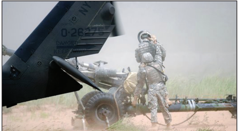
Soldiers get set to hook their 105 mm howitzer to a UH-60 Black Hawk helicopter via a prepared static line on Fort Drum, N.Y., July 17. The Soldiers are assigned to 1st Battalion, 258th Field Artillery, New York Army National Guard; the helicopter crew is assigned to Army Aviation Support Facility 3 in Latham, N.Y. Photo by Sgt. 1st Class Steven Petibone, 42nd Infantry Division.
