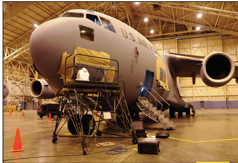
New York Air National Guard Staff Sgt. Brian Burns prepares the nose area of C-17 Tail Number 10188, formerly assigned to Joint Base Charleston, for painting with 105th Airlift Wing markings on Wednesday, October 10. The plane, the second of two extended range C-17s, arrived at the base on Tuesday, Oct. 9. Photo by Tech. Sgt. Michael O'Halloran, 105th Airlift Wing.
