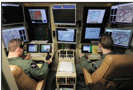
A student pilot and sensor operator man the controls of a MQ-9 Reaper in a ground-based cockpit during training. The 174th Attack Wing created a mock cockpit of the MQ-9 for visitors to the New York State Fair in Syracuse this year. Photo by Tech. Sgt. Ricky Best, 174th Attack Wing.
