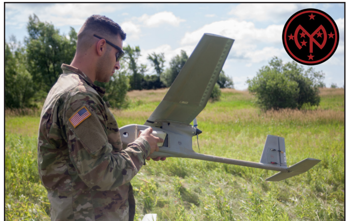
Cpl. Matthew Mena, a field artillery tactical data system specialist assigned to Charlie Battery, 1st Battalion, 258th Field Artillery, prepares an RQ-11B Raven small unmanned aircraft for flight at Fort Drum, July 21. The Raven, a small hand-launched aircraft, is utilized in the field to conduct short range reconnaissance.
