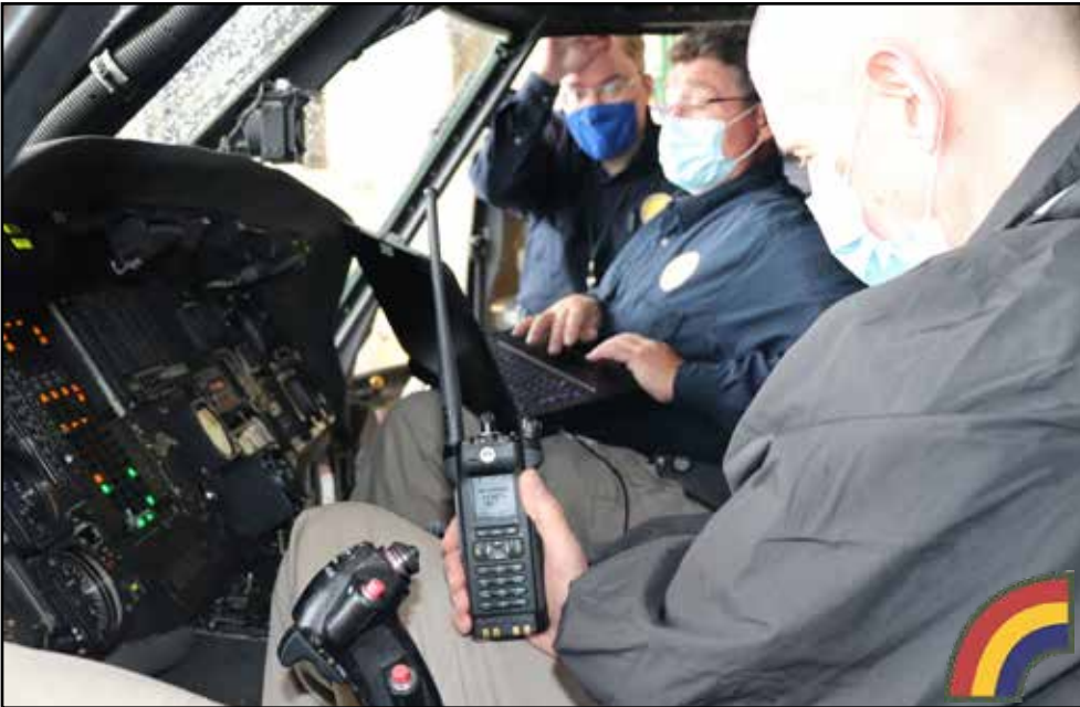
Michael Carl, a radio engineer from the New York State Office of Interoperable and Emergency Communications, uses a portable public safety radio to test the ability of a radio installed in a New York Army National Guard UH-60 to receive signals from a civilian radio while Lawrence Mitchell, another engineer, programs the radio using software on a laptop at the Army Aviation Support Facility in Latham, N.Y. on Sept. 30, 2020. Teams from the office uploaded civilian emergency response channels onto radios on all New York National Guard helicopters. Photo courtesy of Chet Lasalle, New York State Division of Homeland Security and Emergency Services.
