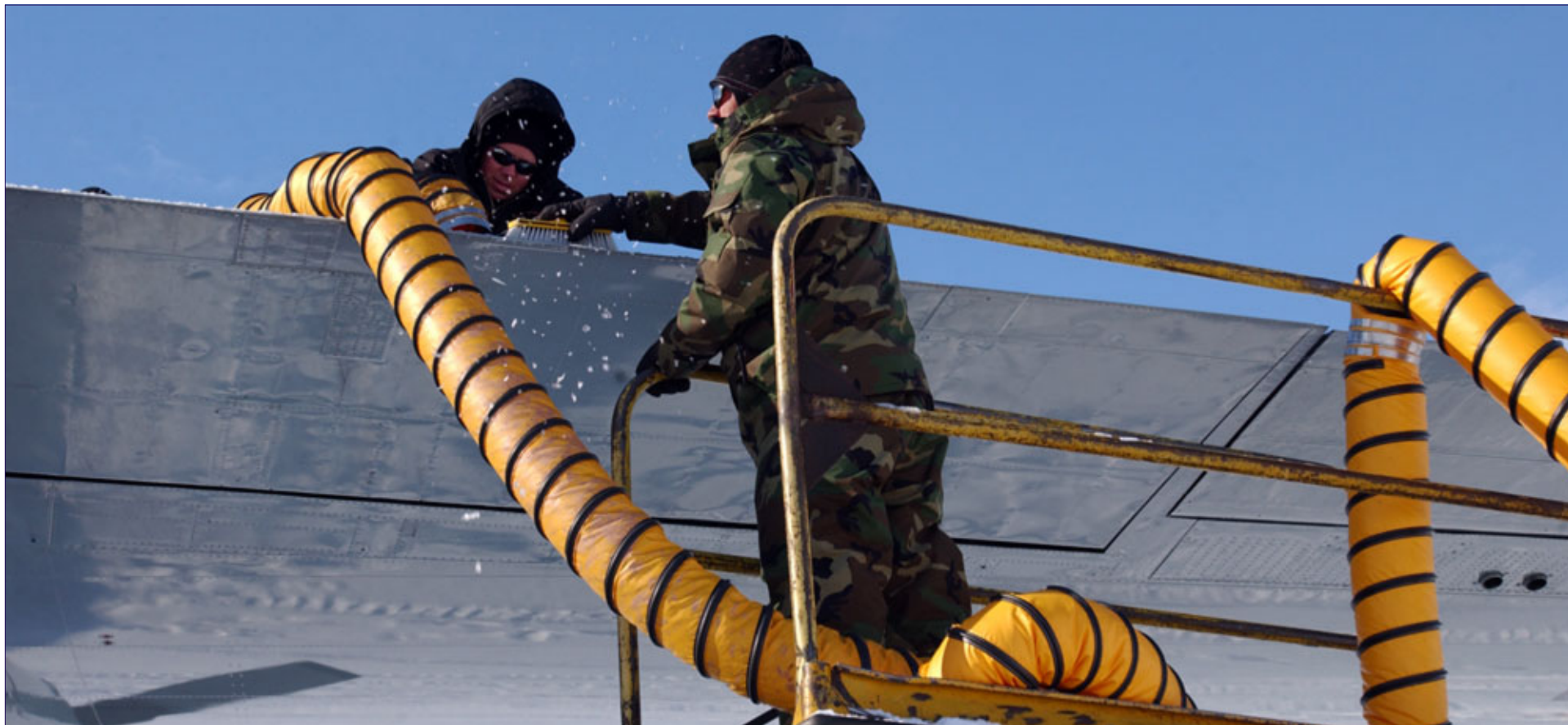
Maintenance Airmen remove ice from a Wing using heater hoses and a brush. Most on-continent aircraft maintenance is performed outdoors under extreme cold temperatures.
