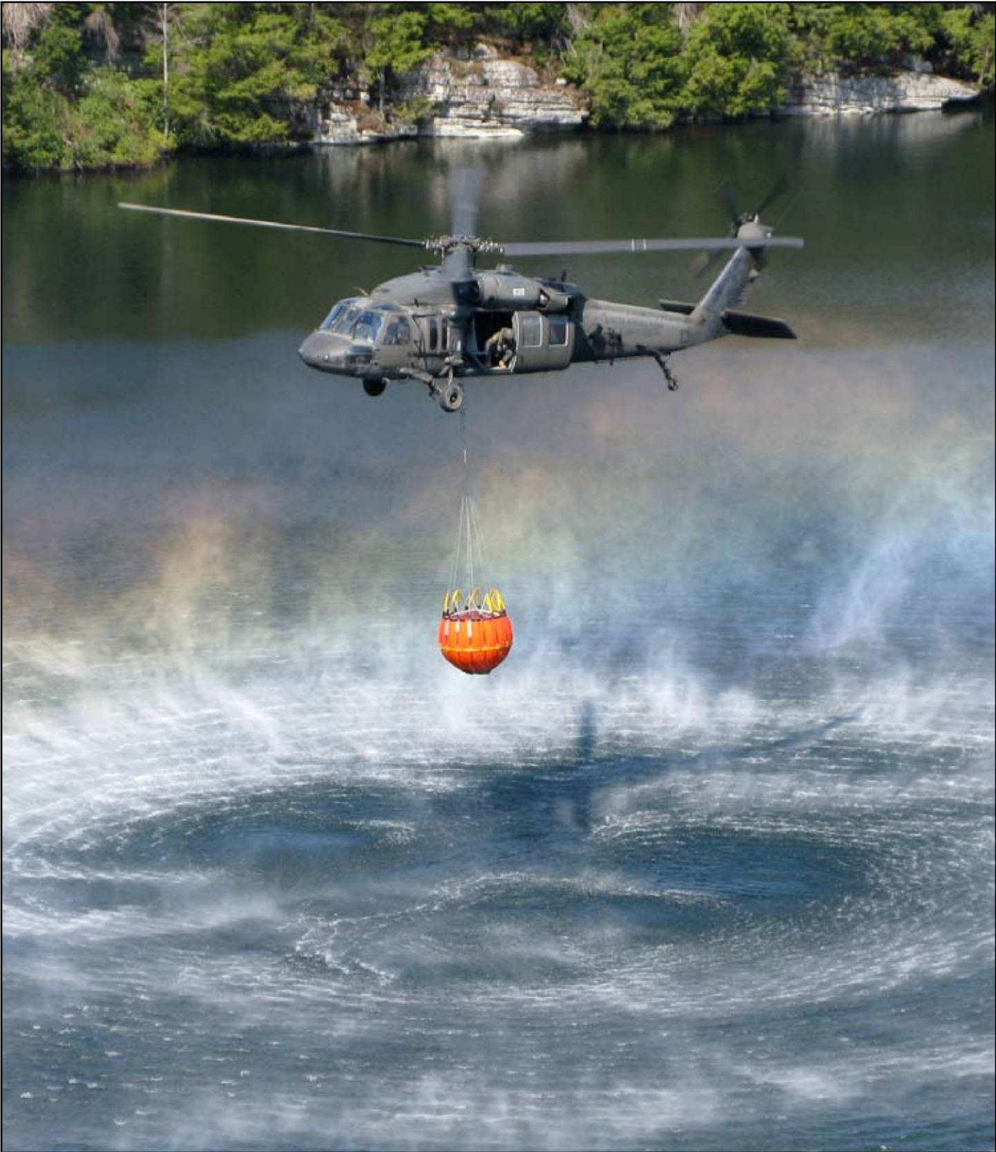
A New York Army National Guard UH-60 Blackhawk fills a 600 gallon "Bambi Bucket" from Lake Awosting in Minnewaska State Park, Ulster County on April 21, prior to making another dump on a 3,100 acre wildfire. Photo by Sgt. Logan Ambrosio.
