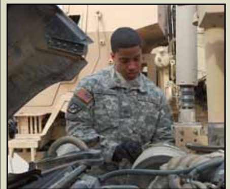
New York Army National Guard Sgt. Darryl Joseph, a light equipment mechanic, checks a transmission belt on a Humvee for rips and tears at Camp Striker, Baghdad, Iraq, Jan. 27.
