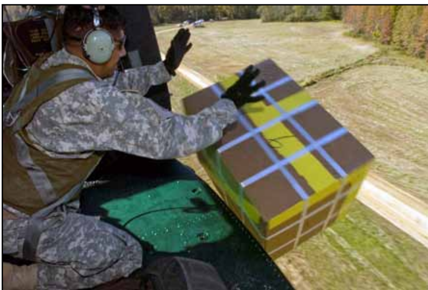
A Soldier pushes a parachute-less free drop package from a helicopter during tests. Called the Freedrop Delivery System, the bundles of up to 150 pounds can be released at 70 knots airspeed from under 75 feet altitude. The Army's chief logistician said he hopes to have the new delivery system in Afghanistan by the end of summer. Photo courtesy of the Aberdeen Test Center.
