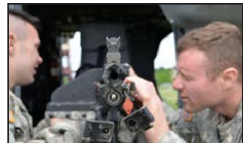
Spc. Mirza Dizinic and Sgt. Ryan Couture assigned to the 3-142nd Aviation mount a M240 to a UH-60 Black Hawk at Fort Drum, N.Y., during aerial gunnery June 2nd, 2018.
