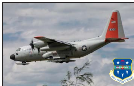
An LC-130 assigned to the 109th Airlift Wing on display at the Paris Air Show on June 18, 2019. The NP2000 propellers, which provide more power and enable fuel economy, are unique and the reason why the wing was invited to attend. Below, An LC-130 comes into land at the Paris Air Show on June 16, 2019. Courtesy photos.
