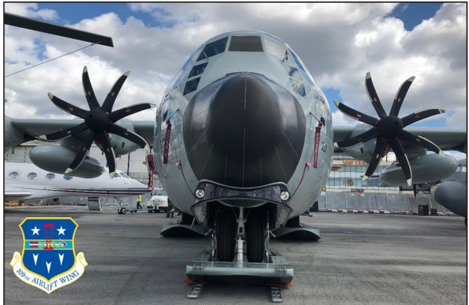
An LC-130 assigned to the 109th Airlift Wing on display at the Paris Air Show on June 18, 2019. The NP2000 propellers, which provide more power and enable fuel economy, are unique and the reason why the wing was invited to attend. Below, An LC-130 comes into land at the Paris Air Show on June 16, 2019. Courtesy photos.
