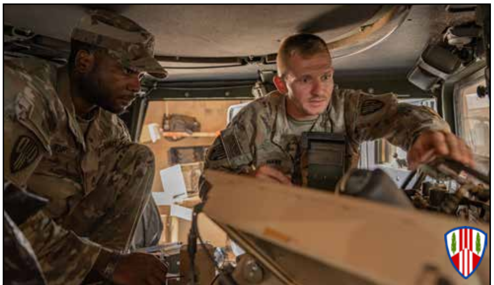
Staff Sgt. Teon Desir, an information technology specialist and Sgt. Michael Mann, a signal support systems specialist with the 369th Sustainment Brigade, install a Joint Battle Command - Platform, or JBC-P during a communications exercise at Camp Arifjan, Kuwait, May 16, 2023. Photo by Staff Sgt. Sebastian Rothwyn, 369th Sustainment Brigade.
