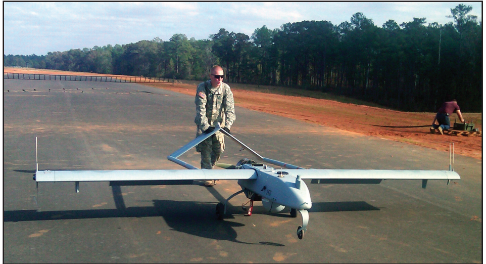
Pfc. Timothy Strong from the 27th Brigade Special Troops Battalion Military Intelligence Company launched the first New York Army National Guard “Shadow” aircraft in December 2010. After recovering the aircraft, he walks the RQ-7 “Shadow” aircraft from the arresting gear in the background back to the maintenance area for servicing.
