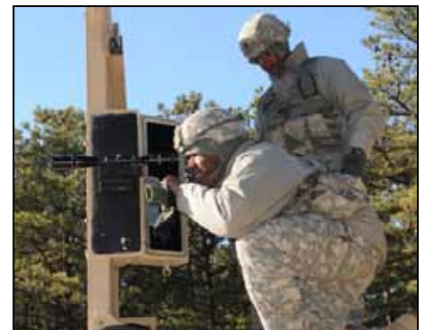
Spc. Jessy Bitwa and Spc. Deshawn Thomas (kneeling) use the bore-sight telescope that is mounted on the AN/TPQ-36 antenna to accurately detect and locate weapons, to align the antenna. The far stake is emplaced at a minimum distance of 100 meters (more than 250 meters preferred) in front of the radar antenna.
