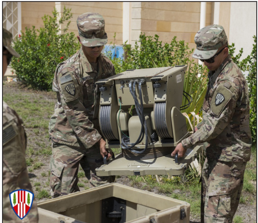
101st Expeditionary Signal Battalion Soldiers Sgt. Abel Burgos-Davila, left, and Spc. Terence Cheung work to assemble the pedestal for an Army secure and nonsecure access point communications terminal at Mohammed Naguib Military Base, Egypt in support of Operation Bright Star Sept. 3, 2018. Photo by Sr. Airman Amanda Stanford, U.S. Air Force.
