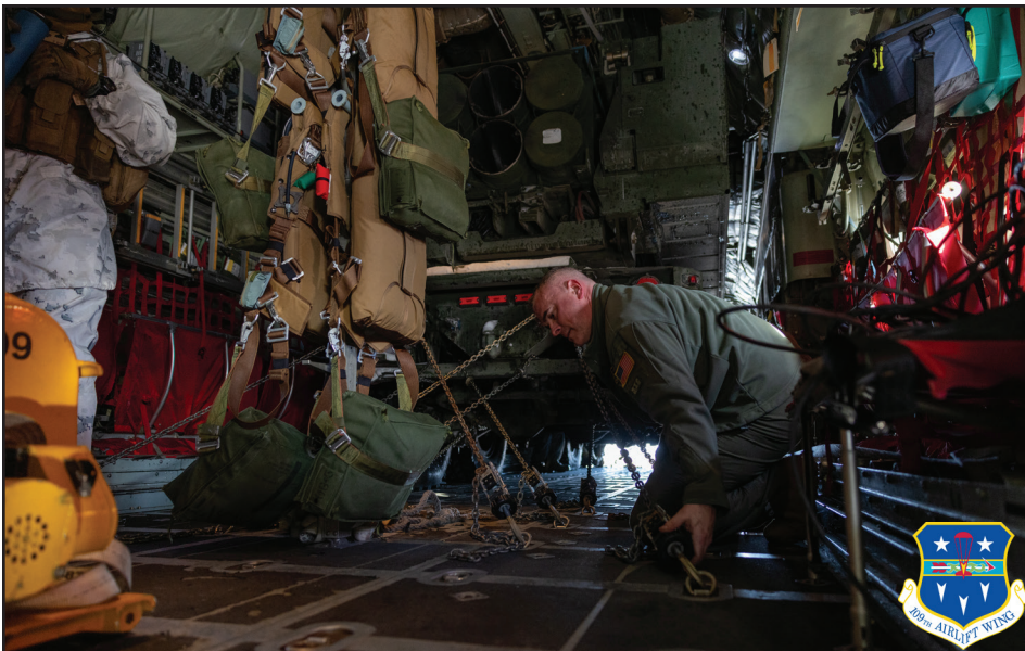
Air National Guard Senior Master Sgt. Dylan Hassis, a loadmaster with the New York Air National Guard 109th Airlift Wing, tightens the tie-down straps securing a High Mobility Artillery Rocket System to a C-130 Hercules aircraft in support of Arctic Edge 24 at Eielson Air Force Base, Alaska, Feb. 24, 2024. Photo by Tech. Sgt. Madison Scaringe, 109th Airlift Wing.
