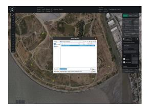
3. If a Flight Plan is already open, a prompt will appear on the right side of the screen to ensure the operator wants to clear the existing file in order to open a new file.
