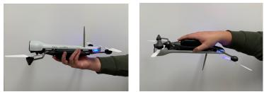
9. Hold the tail end of Vesper up to the screen so the VIO sensor can scan the QR code. A short chime will play to verify that the scan was successful Note: The tail may need to be moved around slightly in order for the VIO camera sensor to successfully scan the QR code; lowering the Vision screen brightness may be helpful.
