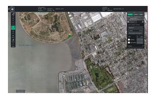
\*Note: A waypoint is a point in three-dimensional space that the drone flies to as part of a mission. Each mission consists of a series of coordinated waypoints. The operator can choose just one, or set multiple, waypoint(s).
